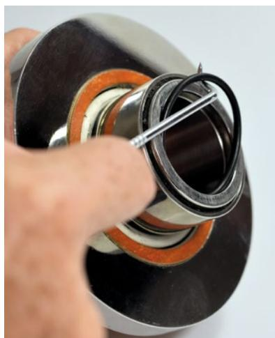
It is sometimes difficult to remove the seal, especially if it has suffered from chemical attack and has adhered to its housing. In order to facilitate its replacement, extraction tools such as those shown in the following image can be used.
